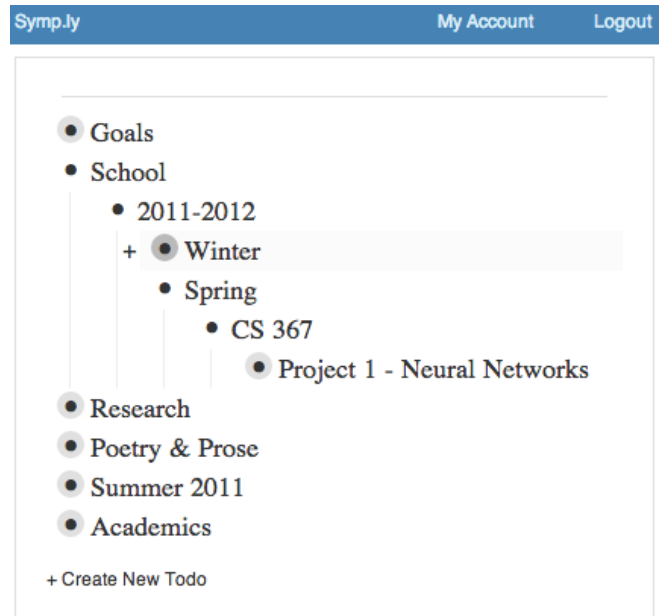
Figure 1. An illustration of the collapsible items of Symp.ly. The items that whose bullets are shaded in gray represent items that are collapsed and have more children nested under them. This allows users to hide items that are not currently relevant to the hierarchical context.
